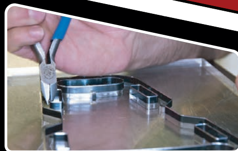
Upper: Steel Rule dies produced by pre-bent metal cutting blades being inserted into notches cut into a wooden base.
